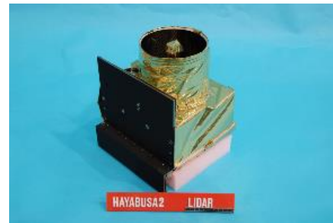
Measures distance between the asteroid and the spacecraft in a range of 30 m–25 km
